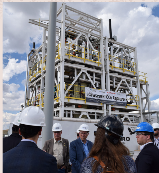
Wyoming Governor Mark Gordon aptly kicked off his Decarbonizing the West chair initiative in Gillette, Wyoming, where workshop attendees got a chance to tour the Wyoming Integrated Test Center – one of the world’s only test centers for carbon capture and utilization technologies using actual coal-based flue gas from an operating coal-fired powered plant. The project in this picture, operated by Kawasaki Heavy Industries and the Japan Carbon Frontier Organization, will demonstrate a novel CO 2 separation and recovery technology using solid absorbents.
