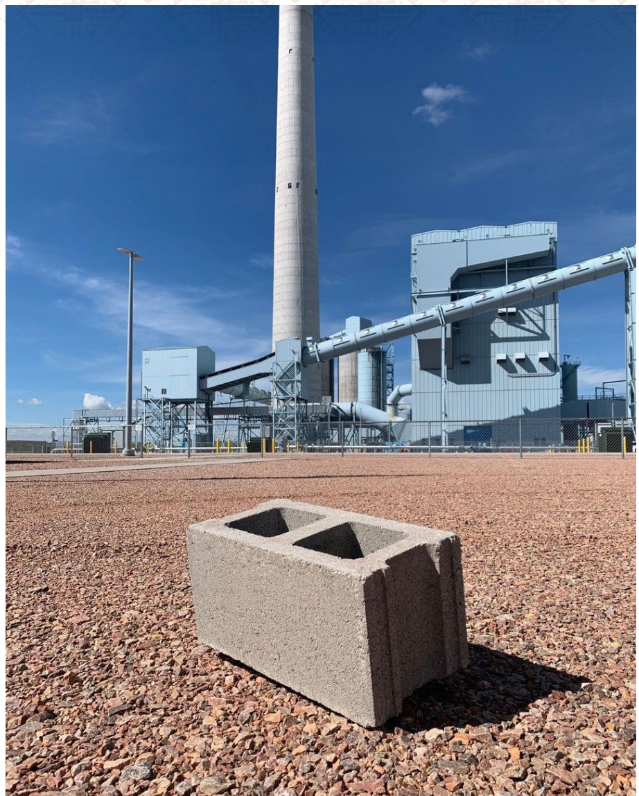
At the Integrated Test Center in Gillette, Wyoming, scientists from UCLA successfully injected carbon dioxide emissions from a coal-fired power plant into concrete, reducing the significant carbon footprint of concrete by up to 100 percent. The concrete blocks created using this technology cost no more to produce than traditional concrete and are now being used in the construction of several municipal projects across the State of Alabama.
